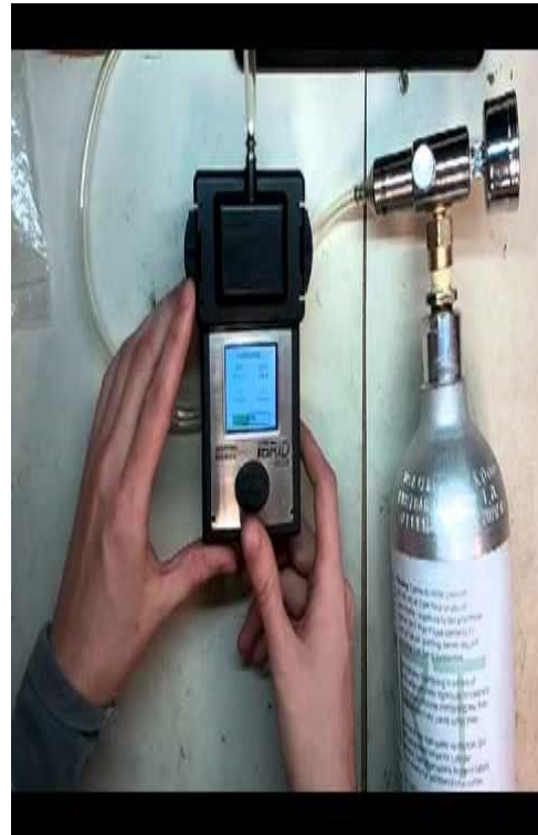
Calibration Set Up for MX 6
